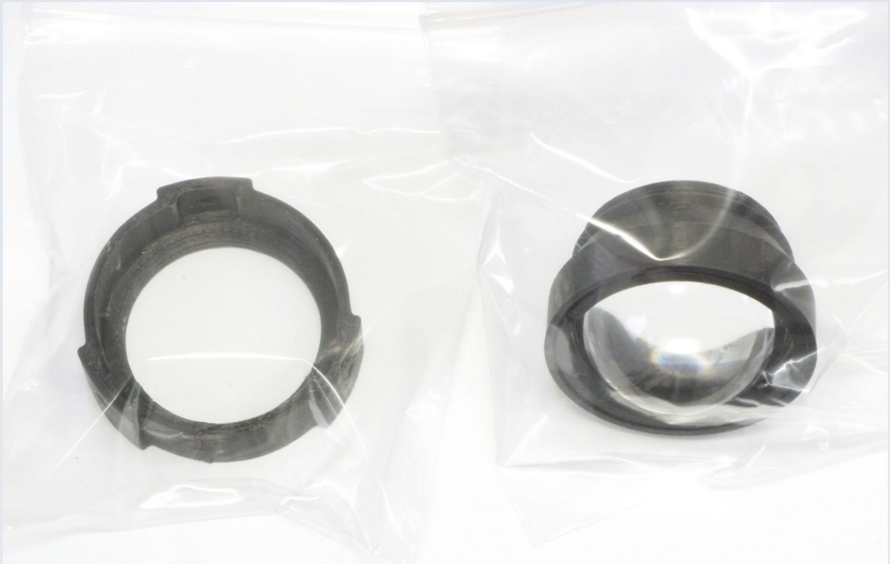
Figure 2. Left: DI_Daylight_Kohler_adaptor. Right: Upper collector assembly and 44 mm lens pre-assembled. This includes the 44 mm lens, DI_Cnd_to_UC, any DI_UC_Spacer models - as many as required to get the position of the lens correct (this is pre-done for you) and a DI_UC_Retention_Cap.
