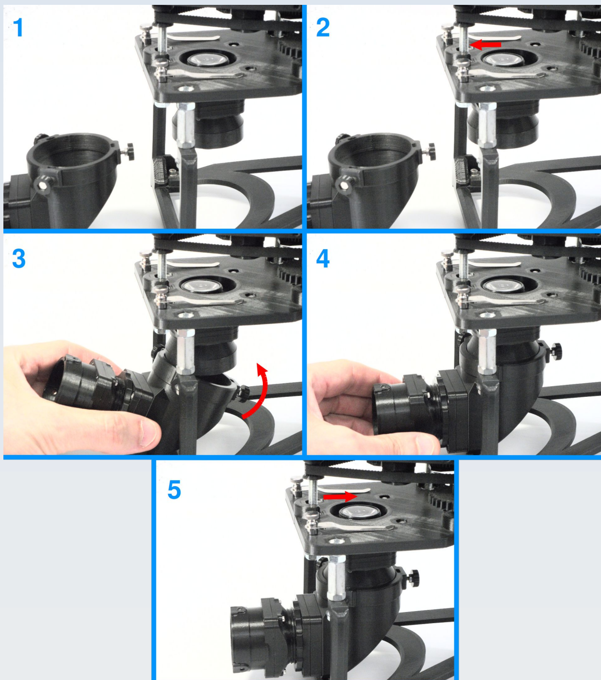
Figure 5. Procedure for connecting the collector mirror block to the upper collector and Abbe condenser without removing the latter structures from the stage. 1. First screw the upper collector assembly to the base of the Abbe condenser then loosen the thumbscrews under the stage that secure the condenser; 2. Slide the condenser / upper collector assembly forward as far as they will go; 3. Hook the collector mirror block onto the upper collector; 4. Secure the collector mirror block to the upper collector with its thumbscrews; 5. Re-centre the condenser and re-tighten its sub-stage thumbscrews. Reverse the process if you need to remove the collector mirror block.
