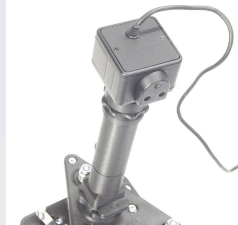
C-Mount camera replacing eyepiece
