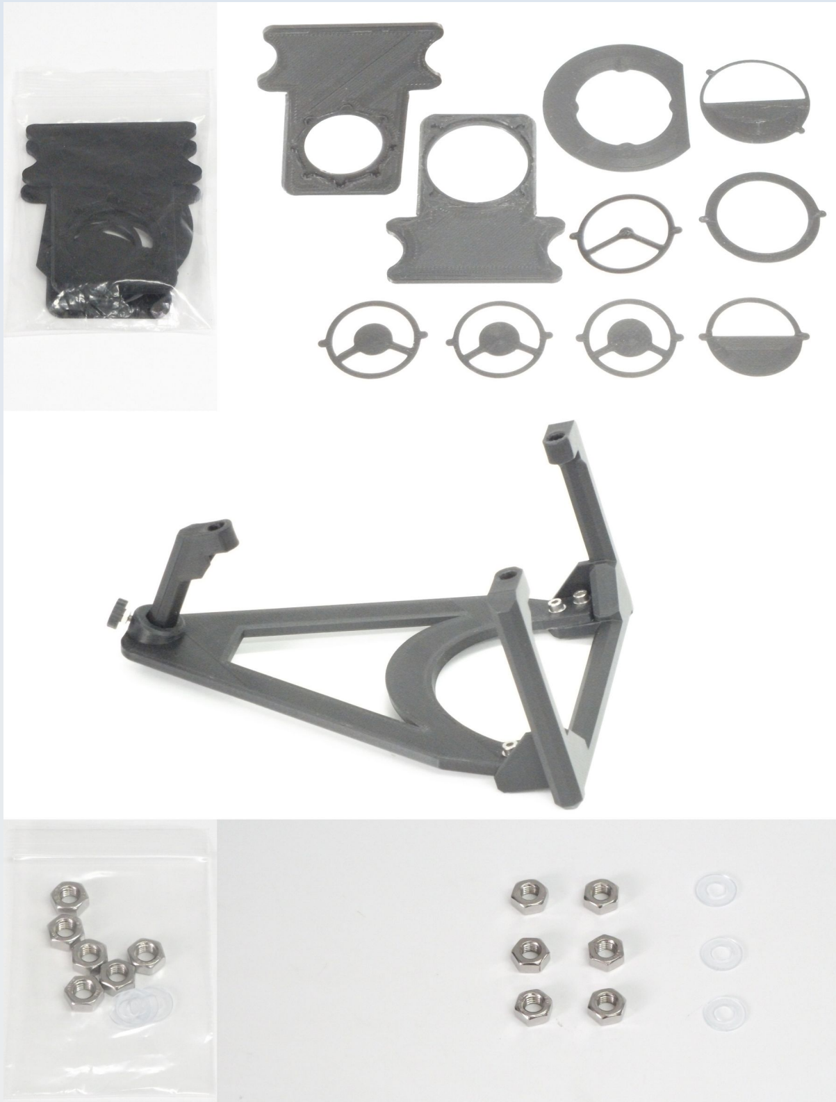
Figure 3. More parts included in the kit. Packs are shown on the left and their contents on the right. Top: The filter pack containing a selection of filters, two filter sliders (the one with the larger aperture is for use with oil immersion objectives) and a spare or additional condenser flange spacer. Middle: The long legs stand system ready assembled for you, Bottom: The 6 M6 nuts and 3 M6 flexible washers used to fix the long legs system to the scope.
