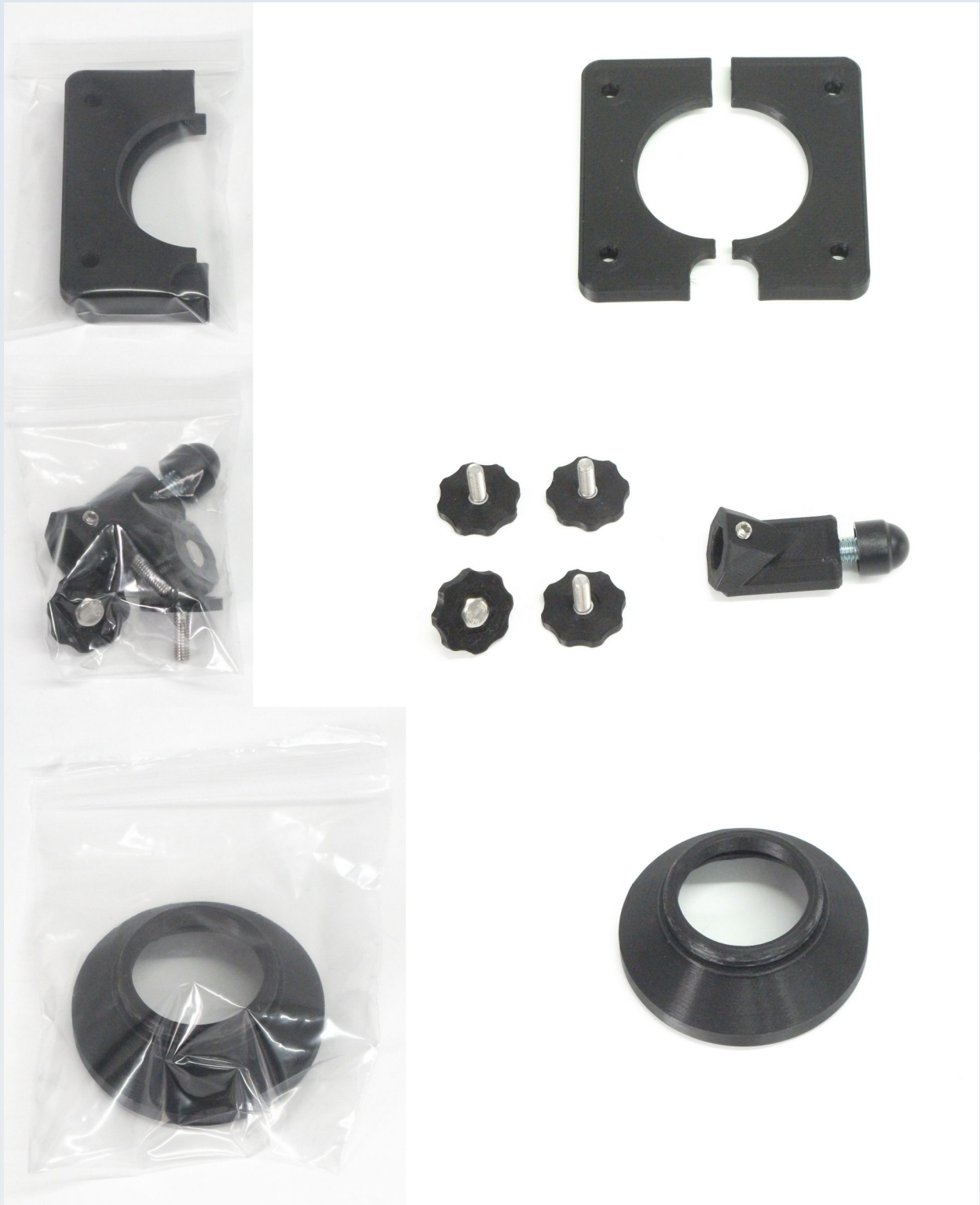
Figure 2. Some other parts of the upgrade kit: On the left are the packs that come in the box. On the right are shown the contents of the packs. Top: The condenser gripper brackets. Middle: The 4 thumbscrews used to secure the gripper bracket plates to the stage and the adjustable hind leg extension for the long legs stand system. Bottom: The condenser mirror holder socket.
