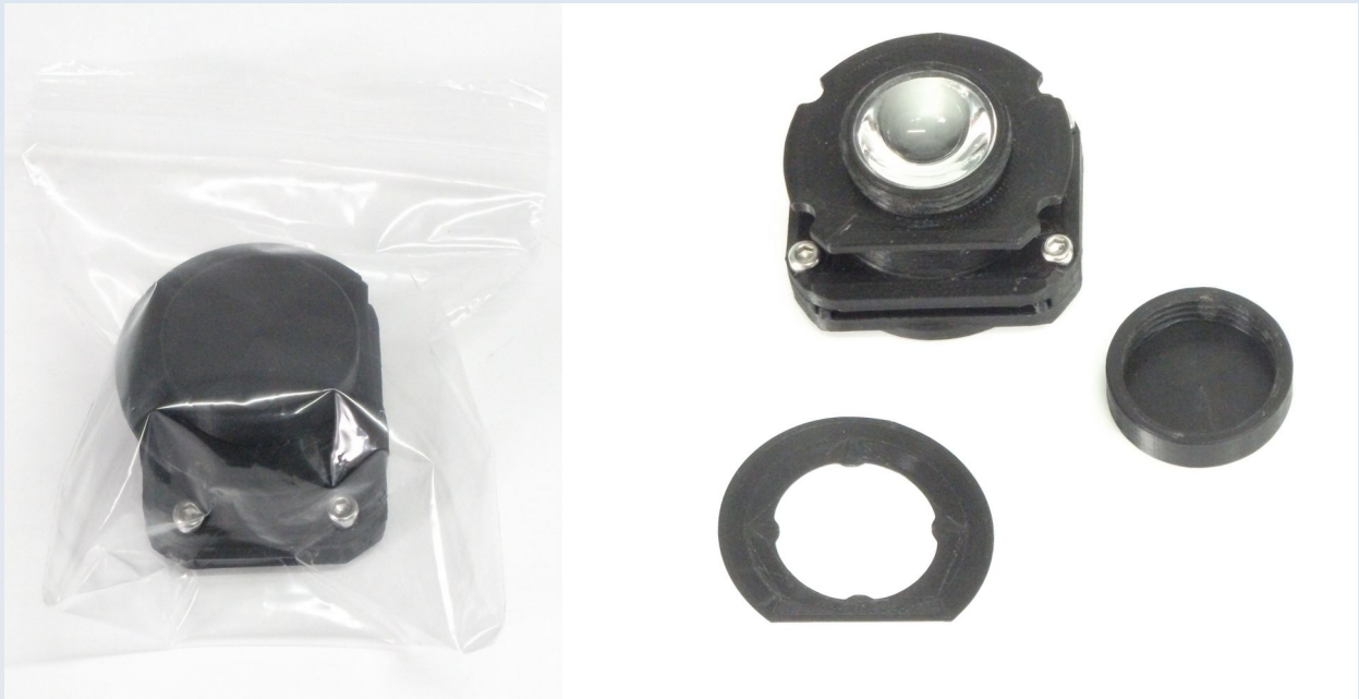
Figure 1. The condenser packet. Packet shown on the left. Parts in the packet shown on the right. Note that these three parts are all fitted together onto the condenser unit and have been removed and separated for the purpose of this illustration. Note that you must remove (unscrew) the protective cap before fitting the condenser to the stage. Note also that the single flange spacer (that is already fitted to the condenser in this packet) is all you need for normal use, so you do not need to attach the other (spare) spacer provided in the 'filters' pack (figure 3).
