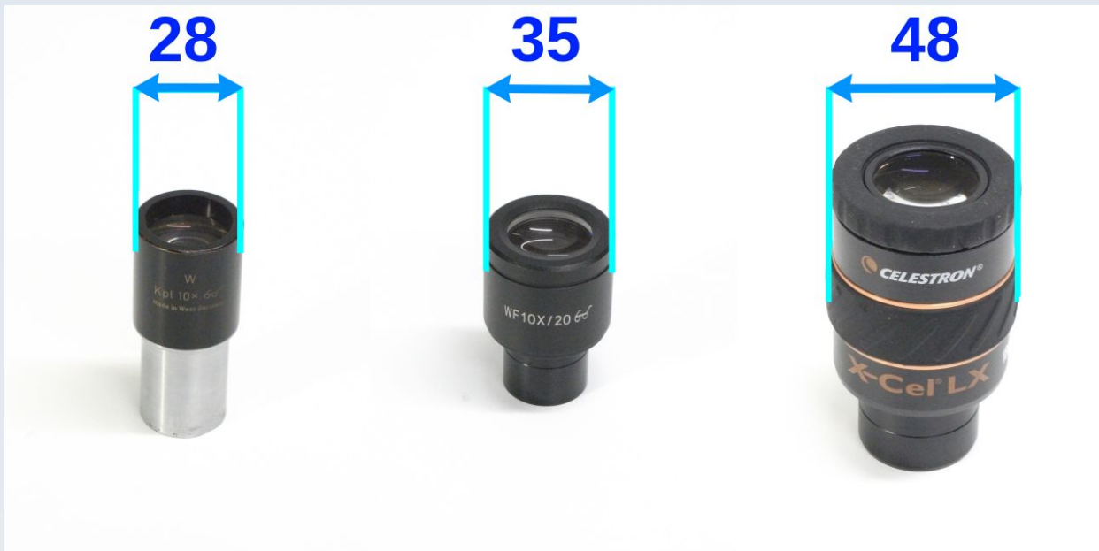
Figure 5.2 Examples of eyepiece maximum outer diameter (in mm) for three eyepieces. Left: Zeiss W Kpl x10, Middle: OptArc WF x10/20, Right: Celestron X-Cel LX 18 mm. Maximum body diameter measurements are shown above each eyepiece (units are mm). The Zeiss will be too small to fit the standard AF51 eyepiece clamp without a special adapter (not supplied). The Celestron will be too large to fit. See text for details.
