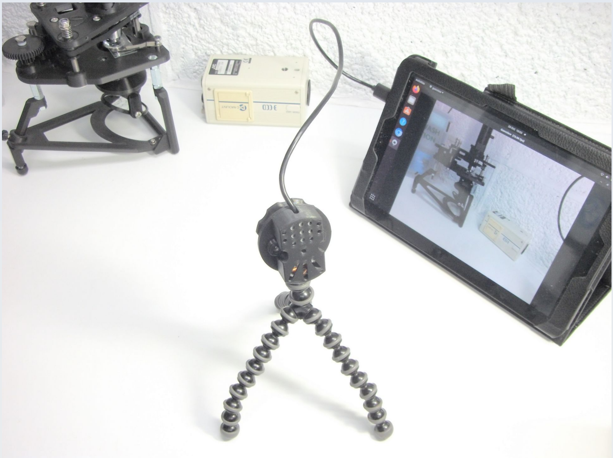
Figure 2.2 The AF51 being used as a 'standard' camera using its in-built lens (no eyepiece or other optics attached). The tripod and tablet computer are optional extras, not included with the AF51 package.
