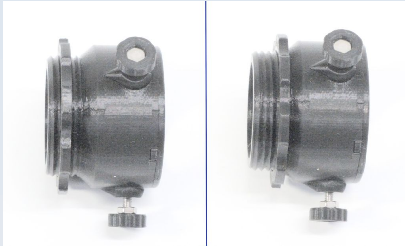
Figure 3.11 The eyepiece clamp and lock nut. You can adjust for the different eye-point / eye relief distances of various eyepieces by means of positioning the locknut at different points along the connecting thread of the eyepiece clamp. Left: The lock nut is near the end for eyepieces with longer eye relief (note there are about 2 full threads between the lock nut and the base of the threaded region). Right: The lock nut is right down the thread for those with shorter eye relief (i.e. 0 threads between the lock nut and the base of the threaded region). This adjustment cannot compensate for eyepieces with very short eye relief and such eyepieces will require a customised adapter to be designed and printed. Such customisations are possible due to the 3D printed nature of the clamp but will need to be done by the user – custom clamp are not supplied with the AF51 as sold by OptArc. For eyepieces with very long eye relief such that even the situation shown on the left does not give sufficient distance, the clamp can be positioned higher up the eyepiece to increase its range.
