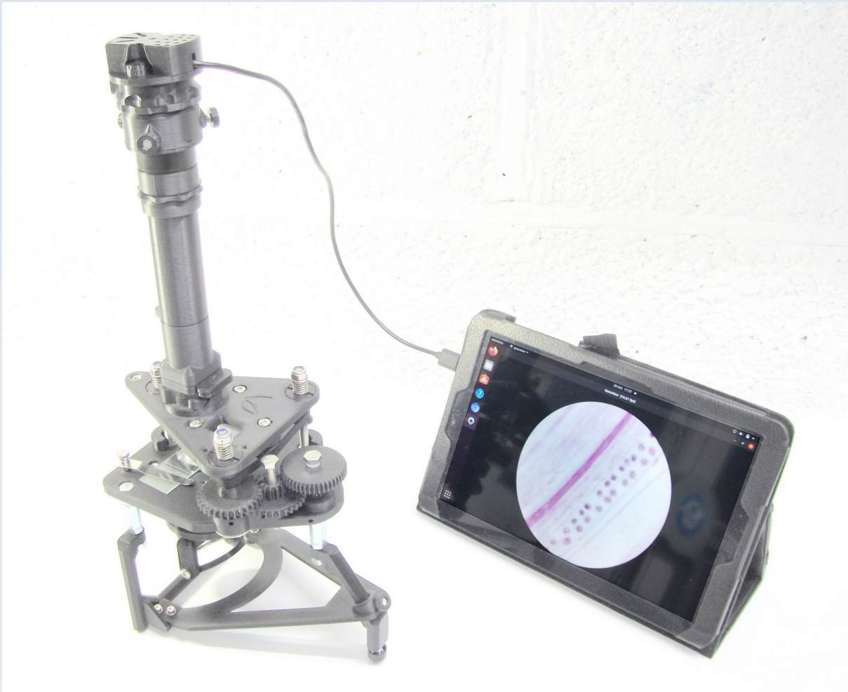
Figure 1.3 The AF51 in use on a PUMA microscope showing a live video image of the specimen under the stage by means of a tablet computer (microscope and computer are shown for illustration, they are not supplied with the camera). Note that the camera shows the complete circular field of view captured by the OptArc x10 WF high eye point eyepiece used in this setup.
