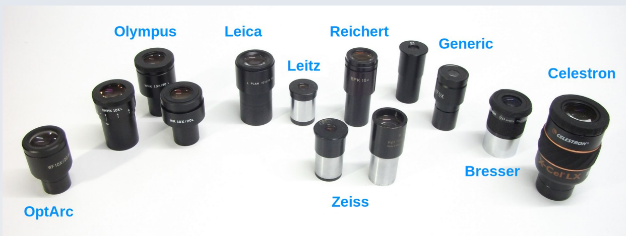
Figure 5.1 The 13 eyepieces tested with the AF51 and results of which are described in this chapter. Not all these will be able to fit in the standard eyepiece clamp provided with the AF51.
