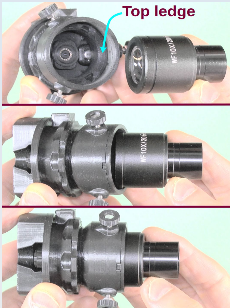
Figure 3.14. Insert the eyepiece body into the clamp till the top ledge of the clamp rests on the top of the eyepiece. This is the default position before starting to make adjustments for best image quality. Once in place tighten the clamp screws to hold the eyepiece steady but take care not to over-tighten the screws to minimise risk of damage to the body of the eyepiece. For some eyepieces with very long eye relief you will need to let the clamp 'ride high' on the body of the eyepiece so that the top ledge of the clamp no longer rests on the eyepiece. See text for details.
