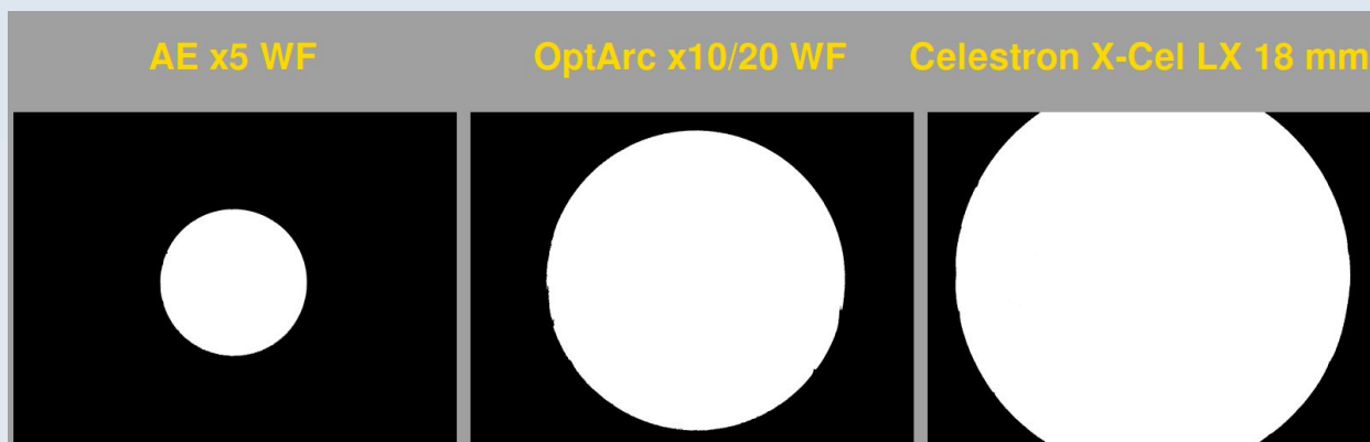
Figure 5.5 The range of field coverage by different eyepieces is very wide. Left: The low cost ‘WF’ x5 eyepiece from Ali Express only uses 0.58 MP of the full 5 MP frame. Middle: The OptArc x10/20 WF eyepiece fills almost the full height of the frame and uses 2.48 MP of the available 5MP. Right: The Celestron astronomical eyepiece has the widest field of view of all those tested – so wide that it overflows the vertical aspects of the frame of the camera to use 3.88 MP of the available 5 MP at the expense of not showing the full field of view. For some uses this will be preferable (e.g. if you want to crop the field of view to a full rectangle). Of these three, only the OptArc eyepiece will be useable with the standard eyepiece clamp that comes with the AF51 camera and the Celestron eyepiece will also need a custom adapter to fit it to the microscope (most biological microscopes do not use a 1.25 inch barrel). Details of field of view usage by the other eyepieces tested are given in table 5.1
