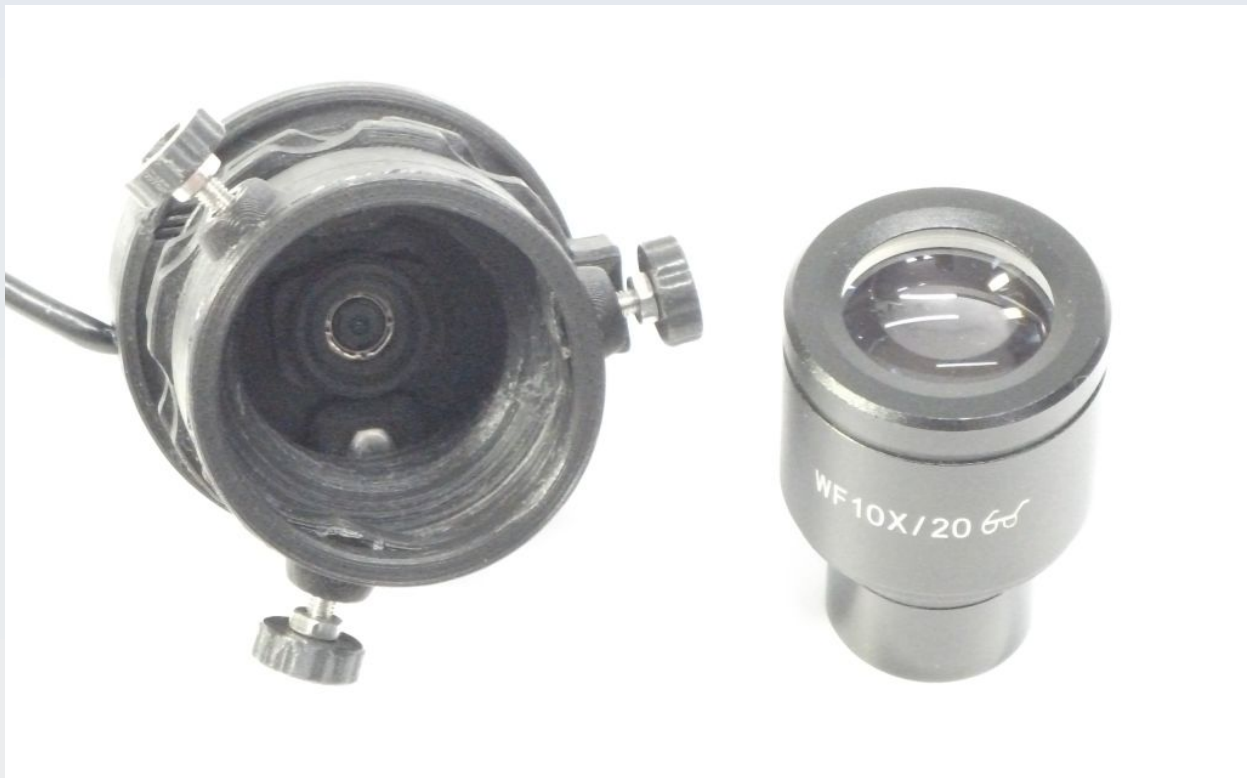
Figure 2.1 The AF51 is recommended to be used with high eye point wide field of view eyepieces such as the OptArc WF 10X/20 eyepiece shown in the figure. Its wide exit aperture and high eye relief allow the AF51 to capture the whole visible field of view with minimal wastage of peripheral pixels (see figure 1.3 for an example of this in use).
