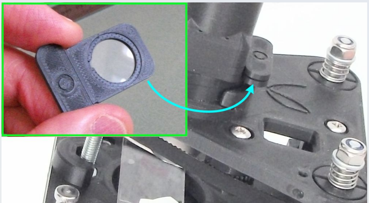
Figure 4. Protect your objectives from falling debris inside the optical tube by making a plain glass filter with a plain 18 mm diameter coverslip in a PUMA filter slider-holder as shown (inset) and keep this 'filter' in the lowest filter slot of your microscope.
