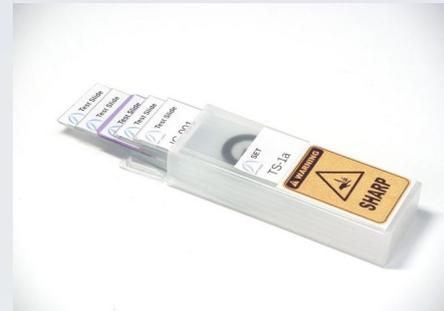
The slides are made of glass so may be damaged if dropped or if leant on and may result in small fragments of glass being chipped off the edges when in normal use due to scraping them against the slide holder system of many microscopes. Please take heed of the safety information and disposal guidance provided in this manual for the safe handling of these specimens.
